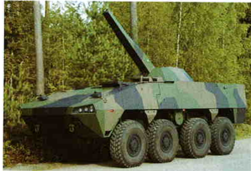
Patria Weapon Systems 120 mm NEMO mortar system integrated onto a Patria AMV 8 x 8 chassis
